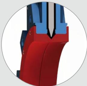
Different coatings can be applied to the gate in order to improve its life and performance onsite. **FCA**'s aim is to avoid issues caused by abrasion, sticky solids and chemical attacks by applying different coatings such as Tungsten Carbide.
